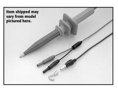
Model 1600A High Voltage Probe MAXIMUM INPUT: 40kV DC or 28kV AC, 50/60Hz. INPUT RESISTANCE:  $1000M\Omega$ . DIVISION RATIO: 1000:1 (into  $10M\Omega$ ).
