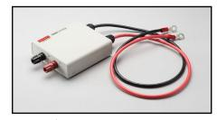
Model 2260B-EXTERM: Extended Terminal Test Leads, 0.7m (28 in.), and terminal box to bring outputs to the front of the instrument or another location. Magnetic base attaches to side of the instrument.
