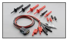
Model 3706-TLK Test Lead Kit: Includes 3706-BAN banana test leads/adapter cable and plugin test lead accessories. Test lead accessories include: 4 spring hook probes, 2 needle test probes, 4 safety plug adapters, and carrying case.
