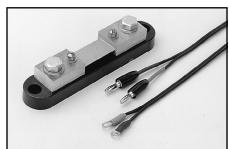
**Model 1651 50 Ampere Shunt:** External  $0.001\Omega \pm 1\%$ , 4-terminal shunt; extends current measuring capability of Keithley DMMs to 50A.
