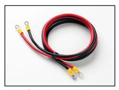
Model 2260-008: Test lead set with lugs, 10AWG, 122m (48 in), red/blue wire pair with #10 terminal lugs on each end.
