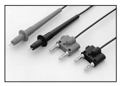
Model 5805 Kelvin Probes: 2 spring-loaded test probes, red and black, 0.9m (36 in) with banana plug termination. Designed to be used with Keithley instruments that measure 4-terminal resistance and in-circuit current. ½-in spacing between pin tips. A package of 8 replacement contacts (P/N CS-551) is available.
