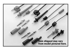
Model 5804 Test Lead Set: Designed to be used with Keithley instruments that measure 4-terminal resistance. Contains: 2 test leads, 0.9m (36 in), red and black; 2 test clips, red and black; 2 plunger clip adapters, red and black; 2 alligator clips with boots (accept standard test probe tip); 2 alligator clips with boots (barrels accept standard banana plugs).
