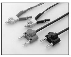
Model 5806 Kelvin Clip Lead Set: 2 clip test leads, red and black, 0.9m (36 in) with banana plug termination. Designed to be used with Keithley instruments that measure 4-terminal resistance. Maximum jaw opening ½ in. A package of 8 replacement elastic bands (P/N 5806-306B) is available.
